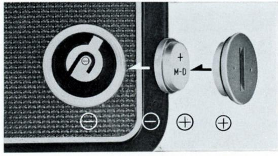
2 Place the mercury battery in the Battery Compartment, make sure the (-) side faces inside. The lid will fail to close if the polarity of the battery is reversed. One replacement of a mercury battery provides sufficient power to work the meter for a period of about two years under normal Use. However, it is advisable to check the battery once
