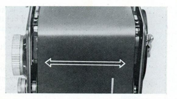
7 Continue winding the film until the "start" mark on the film leader paper lines up with the green triangular (▲) "start" mark for 120 film on the body side.
