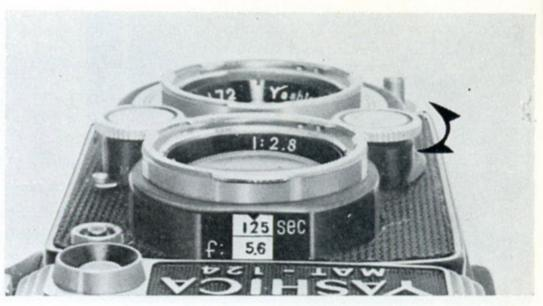
2 Center the desired shutter speed in the Shutter Speed Indicator Window by turning the Shutter Speed Control Dial. The exposure meter pointer in the Exposure Indicator Window is coupled to the shutter mechanism and will shift in either direction when the shutter speed is adjusted.
