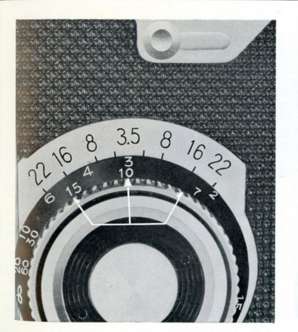
The depth of field for a given aperture and cmera-tosubject distance can be read off the depth-of-field scale around the Focusing Knob. By checking this scale, you can easily determine before shooting the extent over which the objects will appear sharp and clear.
