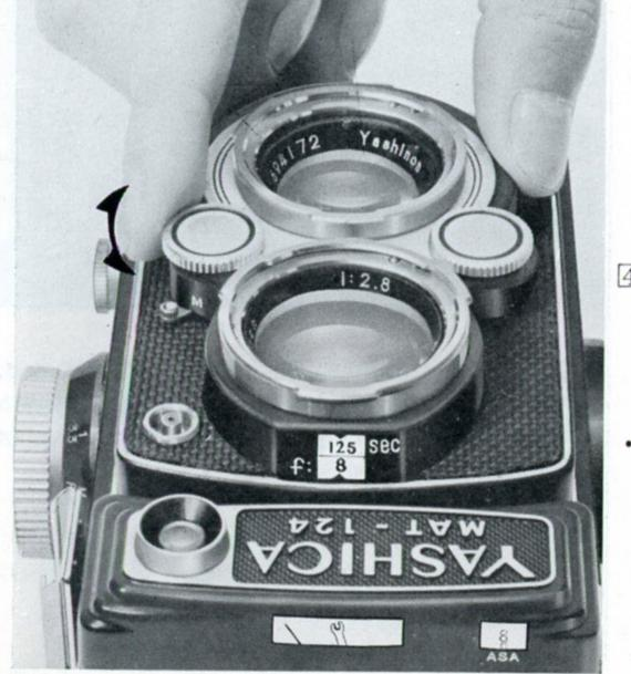
Turn the Aperture Control Dial and coincide the yellow follower needle (coupled to the aperture mechanism) with the red meter pointer (coupled to the shutter mechanism), both visible in the Exposure Indicator Window.
