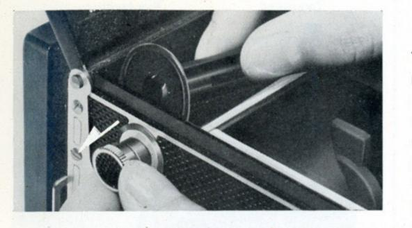
To minimize the trouble in loading your next film, it is advisable to take out the empty spool from the lower film chamber and to set it in the upper chamber immediately after unloading the exposed film.
