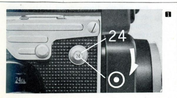
When the figure "24" appears in the exposure counter window, it signifies that the full length of the film has been exposed. Another wind of the crank-handle will bring out the
