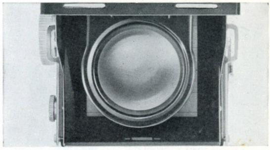
To focus, turn the Focusing Knob while observing the image of your subject produced on the Focusing Screen. After focusing, compose your picture.
