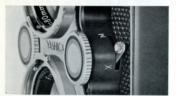
Always set the Flash Synchronizer Selector to "M" with M-class bulbs.
