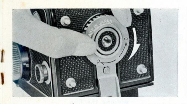
Then, close the Back Cover and turn the Back Cover Locking Ring toward "C" (Close) while pressing the cover. (When closing the Back Cover, see that the lug on the body rests properly in the slot on the Back Cover Latch.)
