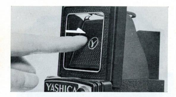
Your YASHICA-MAT 124 features a magnifying lens for critical focusing which springs up into position when the sportsfinder frame section of the Focusing Hood is pushed in slightly.
