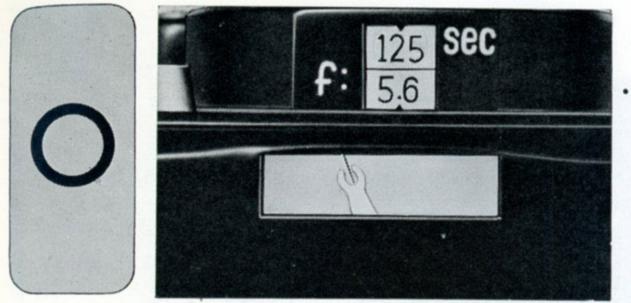
When the yellow follower needle (Y) perfectly coin-cided with the meter pointer(I), it signifies that your YASHICA MAT 124 is set for correct exposure. The proper combination of the shutter speed and aperture is shown in the Shutter Speed and Aperture Indicator Windows.
