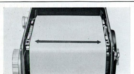
Continue winding the film until the "start" mark on the film leader paper lines up with the red triangular (▲) "start" mark 220 film on the body side.
