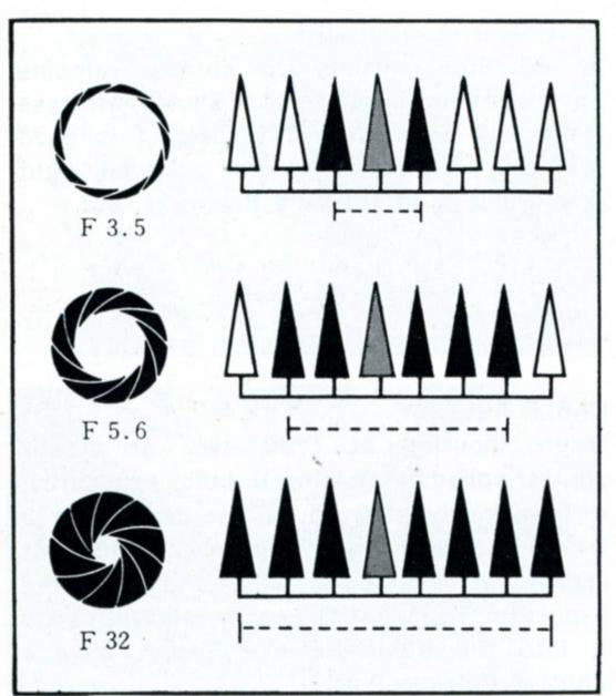
The depth of field is the range in the foreground and background over which all objects appear acceptably sharp when the camera is focused on a given subject. The extent of the depth of field varies with the aperture of the lens and the camera-to-subject distance.
