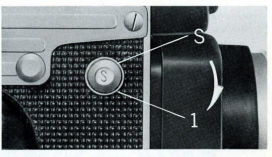
9 The letter "S" appears in the Exposure Counter during the film loading operation. After closing the Back Cover, wind the crank-handle until the figure "1" appears in the Exposure Counter window.
