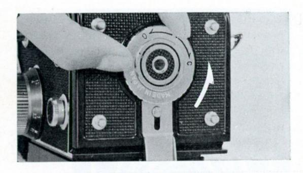
Open the Back Cover by turning the Back Cover Locking Ring in the direction of "O" (Open).
