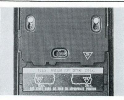
When loading a 220 film (24 exposures), align the red 24 mark on the film pressure plate with the red 24 EX indication and mount it in position in the same manner as explained above.
