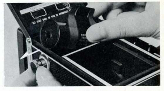
Pull out the Upper Spool Holder Knob and take out the exposed film from the film chamber. Paste the seal to prevent recoiling and wrap the film in light-proof paper.
