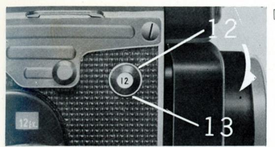
When the figure "12" appears in the exposure counter window, it signifies that the full length of the film has been exposed. Another wind of the crank-handle will set the exposure counter between "12" and "13", but continue winding until the crank-handle turns freely without tension.
