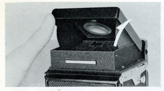
Set the Focusing Hood upright by lifting it up all the way. The Focusing Screen feature eight red lines which facilitate picture composition.
