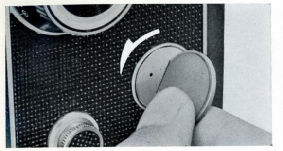
1 Open the Battery Compartment Lid by using the edge of a coin.
