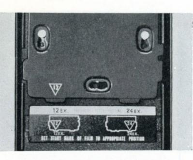
3 When loading a 120 film (12 exposures), position the green 12 mark on the film pressure plate so that it aligns precisely with the green 12 EX indication. Set the pressure plate so that its hole (\*\*) rests properly on the stud and slide it toward the smaller side of the twin hole to mount it in position.
