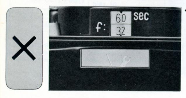
If the yellow follower needle fails to align with the meter pointer, alter the shutter speed setting by turning the Shutter Speed Control Dial in either direction. If the two needles fail to match even when both the shutter speed and aperture settings are changed, it means that correct exposure cannot be obtained under the prevailing light condition. In such a case, the use of a flash unit is advised.
