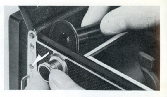
Pull out the Upper Spool Holder Knob and place the empty spool in the Take-Up Spool Chamber. After the Takeup Spool is set properly in the camera, return the Spool Holder Knob to its original position.
