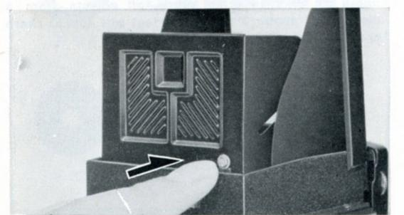
To close the Cover, push the Release Button on the back of the Focusing Hood.
