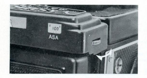
Turn the ASA Film Speed Setting Ring until the figure denoting the ASA rating of the film in use aligns with the red indicator in the ASA Film Speed Indicator Window.
